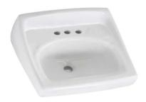
American Standard Commercial Sinks can be found wherever durability, dependability and beauty are on call. The Lucerne wall-hung sinks have a front overflow, D-shaped bowl, and self draining deck area with contoured back and side splash shields. The wall-hung Lucerne Bathroom Sink shall be made with a single center hole, four inch center, or eight inch center faucet configuration with or without front overflow. Sink shall have a width of 20-1/2 inches and a length of 18-1/4 inches.
