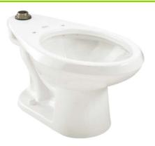
The floor-mounted elongated flushometer bowl shall be made of vitreous china. Product shall be 26" in length, 14" in width, and 15" to 16-1/2" in height when installed on a wall-hung carrier by others. Product shall have a 12" x 10" water area. Product shall have 2-1/8" (54 mm) glazed trapway, and a 1-1/2" top or back spud. Product shall be available with or without bedpan lugs and with or without the EverClean surface.
