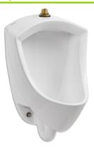
The wall-hung urinal shall be made of vitreous china. Product shall be 22-5/8" in length, 14-5/16" in width, and 14-7/16" in depth. The washdown urinal operates in the 0.125 gpf to 0.50 gpf range. Product has a 3/4" inlet top spud, 2" outlet spud, and includes two wall hangers. Optimized chinaware contours provide superior splash protection.
