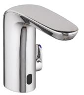
Step into the next generation of Selectronic products by American Standard with the clean, sleek NextGen faucets. The NextGen Selectronic faucets showcase American Standard's exclusive new ASSE 1070 certified SmarTherm Safety Shut-Off that automatically protects the user from scalding. The integrated electronics locates the sensor, battery and solenoid valve in the faucet spout and eliminates the need for a control box. The simple, integrated design allows for easy installation and maintenance.
