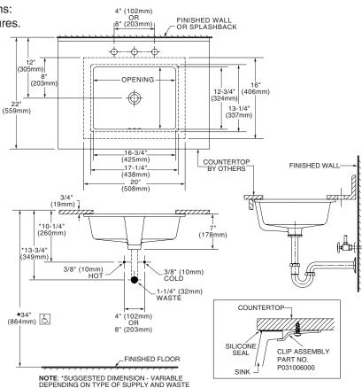
\* To comply with ADA standards, overflow hole must face back.
